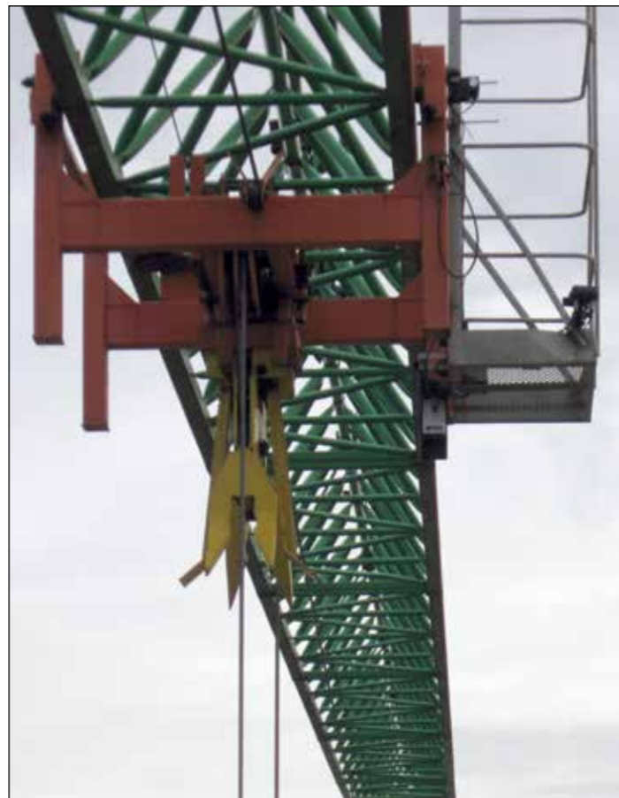
Orlaco Quick Fit Set with Battery pack and Camera AFZ, Orlaco Autocontact and the Orlaco Spectrum Scanner mounted on the trolley of a tower crane.
