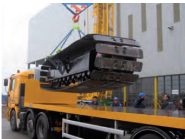
Lifting track off trailer
